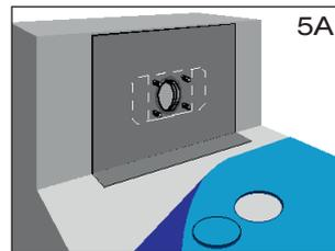
1.5 Unroll the **bituminous** or **plastic** vapour barrier sheet. Make a circular cut (Fig. 5 or 5A) in the vapour barrier sheet in the region of the sliding flange.
