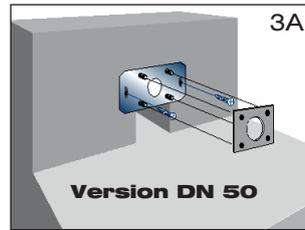
1.3 Fasten the sliding flange (DN 70 and DN 100 versions, with connecting sleeve rolled together or sliding flange (DN 50 version with compression seals) using a screwdriver for slotted screws (Fig. 3 or 3A).
