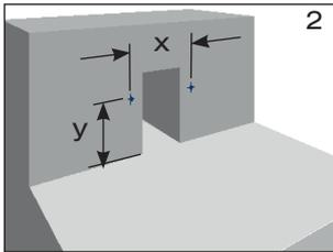
1.2 Make 10 mm diameter holes for the sliding flange with the connecting sleeve or the sliding flange with compression seals for connecting the vapour barrier according to the details specified in Table 2 (Fig. 2).
