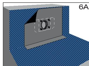
1.6 A bitumen primer must be applied to the slab and wall when bituminous vapour barrier sheets are used (Fig. 6 or 6A).
