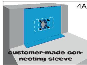
1.4 Spread the connecting sleeve ready-mounted at the factory (DN 70 and DN 100 versions) or the connecting sleeve made by the customer (DN 50 version) consisting of **bitumen/EPDM compound** or of **plastic**, and attach it to the substrate (Fig. 4 or 4A). Do not allow creases to form. On the DN 50 version make 14 mm holes in the connecting sleeve with a hole punch for the threaded bolts to pass through. The loose flange can be used as a template.
